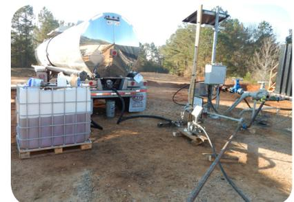
Formulation truck directly connected to injection pump for in-line mixing and direct injection of the foaming formulation.
